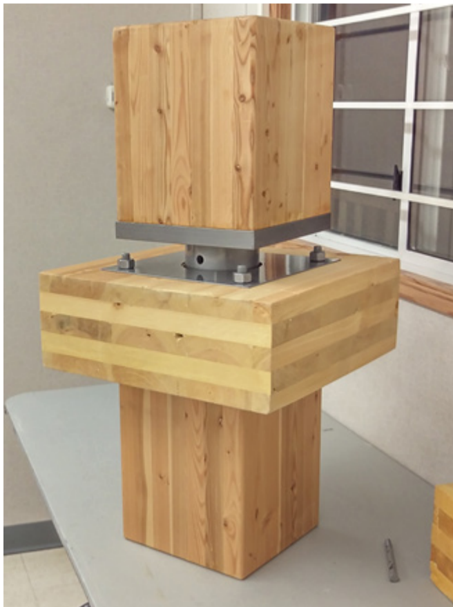
Figure 2.8 CLT floor panel detail with glulam columns above and below from UBC Brock Commons demonstration (Photo: D. Moses)
