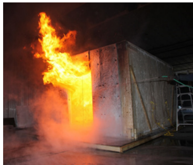
Figure 3.12. During fire test on CLT room with bedroom furniture at Carleton University.
