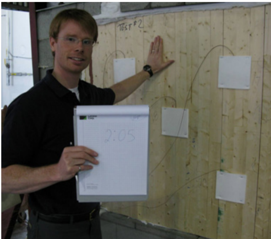
Figure 3.6. Photo during fire-resistance test on 3-ply CLT wall panel after 2-hours and 5-minutes of fire exposure with the unexposed surface still relatively cool.
